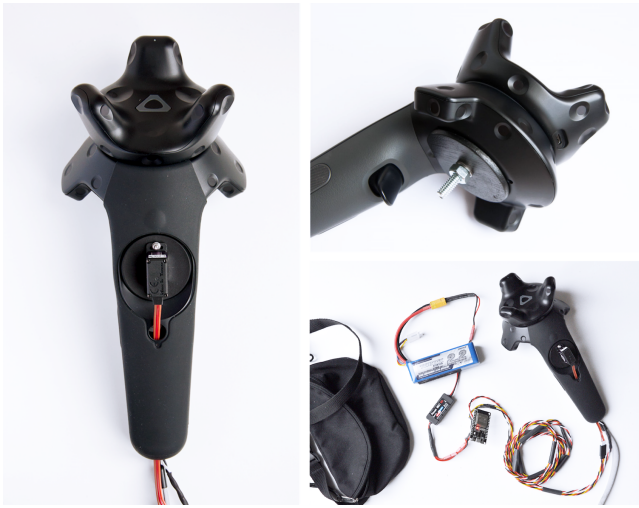
Figure 3: (left) Our haptic VR controller Triggermuscle. (top right) Attachment of the HTC Vive tracker to enable spatial tracking. (right bottom) Electronic components (MCU, the battery, and the BEC) are carried in a small bag.
